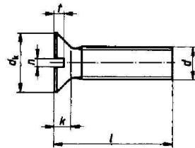
Slotted countersunk head screws
