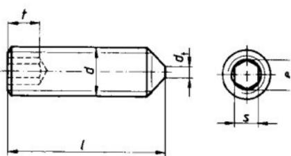
Hexagon socket set screws with cone point
