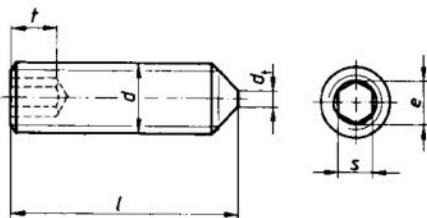
Hexagon socket set screws with cone point
