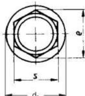
Self drilling screws with hexagon head and flange
